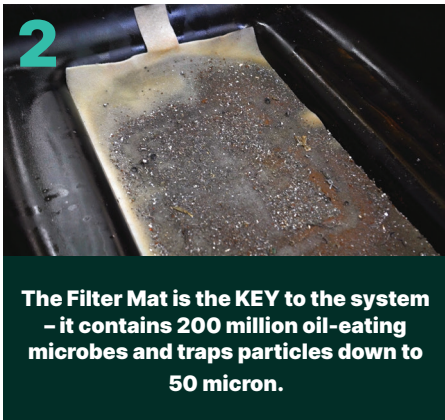
Oil and grease are washed off the dirty part and flow through the Microbial Filter Mat in the sink into the ROWasher tank.
